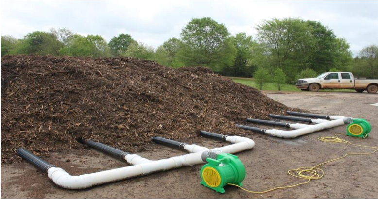
Figure 3 - actively ventilated compost heaps.
